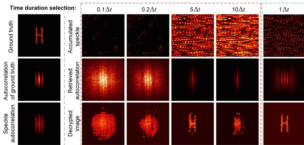
**Fig. 9** Cracking resistance test with wrong time duration selection (in the red dash box). The correct process with a proper time duration selection is also presented in the green dash box.
