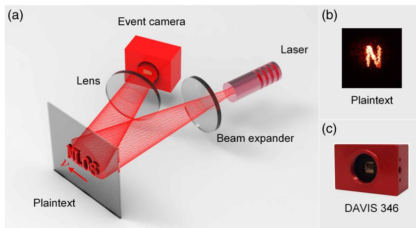
**Fig. 2** Neuromorphic encryption system. (a) The optical configuration. (b) An encrypted letter “N” is made with a diffuse metal surface, captured with frame-mode and a focusing lens. (c) An event camera is employed as the neuromorphic sensor to collect the encrypted data.
