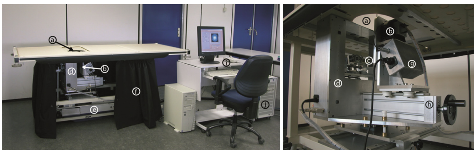
Fig. 1 The Twente photoacoustic mammoscope. (a) Aperture to insert breast. (b) Ultrasound detector matrix. (c) Glass window. (d) Scanning system compartment. (e) Q-switched Nd-YAG laser operated at 1064 nm with 10-ns pulses. (f) Laser safety curtain that is drawn around the instrument during the measurements. (g) Interface electronics between detector and computer. (h) Linear stage carrying detector matrix driven by hand wheel to apply mild compression to the breast. (i) Laser remote control unit. (j) Laser power supply. Image adapted from Ref. 21 with permission.
