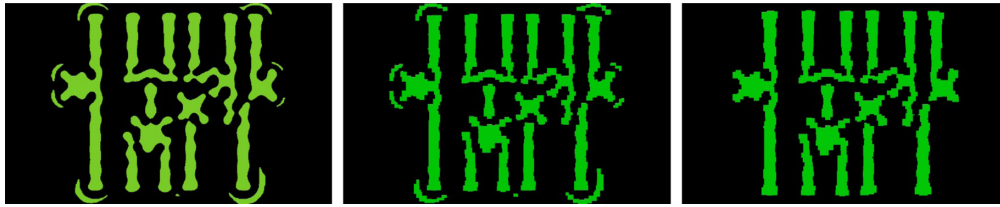
Fig. 1 The original ILT mask patterns shown in the luminescent ILT paper are curvilinear. 9
