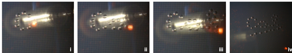
Fig. 12 Snapshots of droplets moved to form the University of Berkeley, California Cal logo. 65 nL total volume droplets dispensed by a droplet-on-demand system from above to the right side on the co-planar OEW device's active region and positioned on the device surface via OEW to form the Cal logo. The 3- \mu\text{m} metal line width and 300- \mu\text{m} metal pitch size OEW device was actuated at 44 V_{pp} and 10 kHz.
