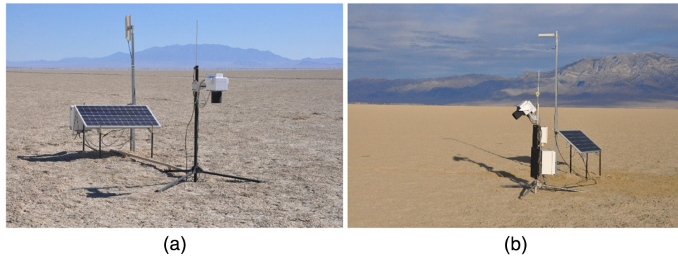
Fig. 1 (a) GVRs at RadCaTS in a nadir-viewing configuration and (b) GOES 16 viewing configuration.
