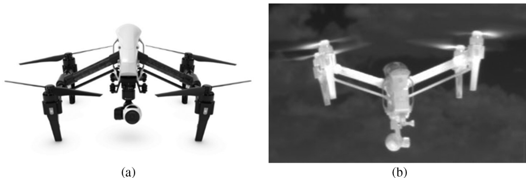
Fig. 2 (a) UAV2 DJI Inspire 1 model and (b) MW image.
