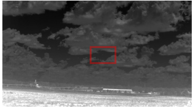
Fig. 3 Background with ROI. The flight path of the UAV went directly from the sensor to this clear region in the clouds. The background of the UAV is always this clear region.
